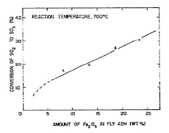
Fig. 4. Conversion of SO<sub>2</sub> to SO<sub>3</sub> at 700 °C as a function of the Fe<sub>2</sub>O<sub>3</sub> content of fly ash.
