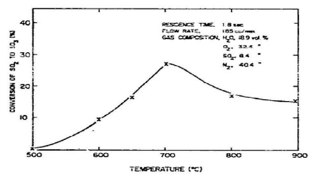
Fig. 3. Conversion of  $SO_2$  to  $SO_3$  in the presence of fly ash as a function of temperature.
