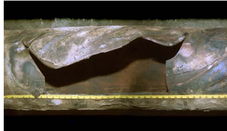
Fractured gasoline line— undetected damage
