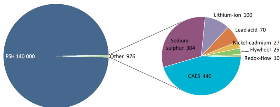
Figure 3 Current global installed grid-connected electricity storage capacity (MW), (IEA, 2014)
