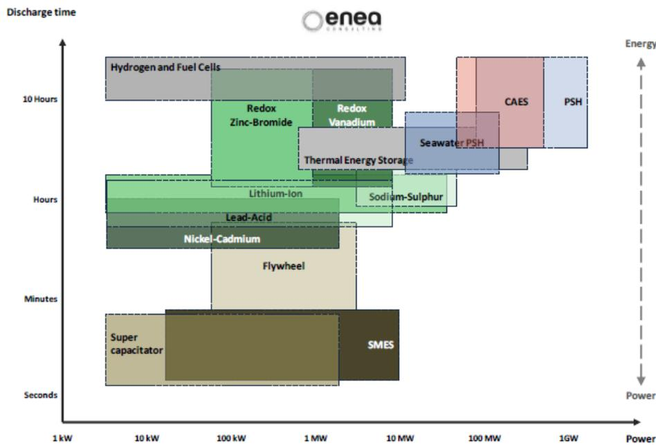
Figure 1 Energy storage according to discharge time and typical power (ENEA, 2012)
