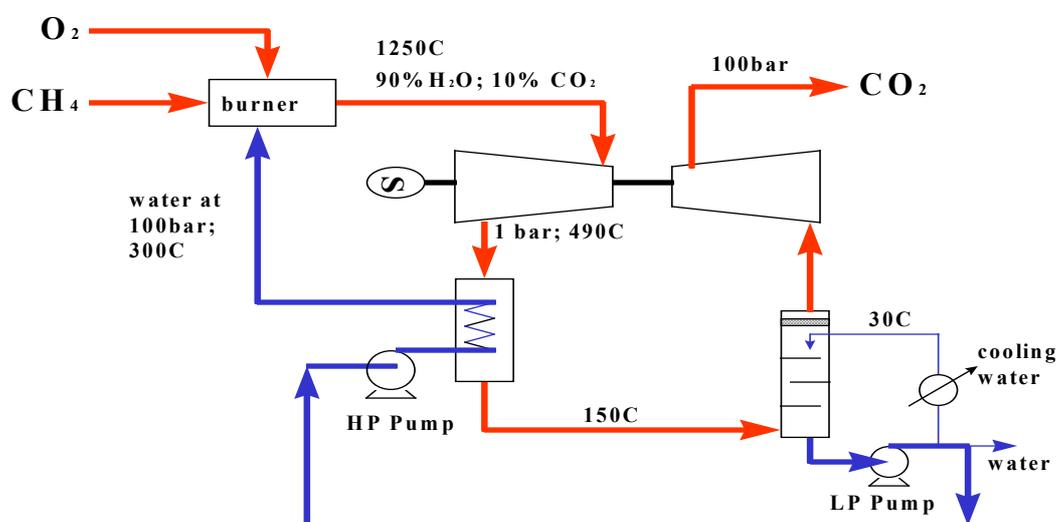
In the process, natural gas (or any other fossil fuel) is burnt in a combustor. High-purity oxygen produced in an ASU is used as an oxidant. The reaction temperature is controlled by the injection of (liquid) water which is recycled after being recovered from the process flue gas. An expansion turbine is used to generate electricity.
