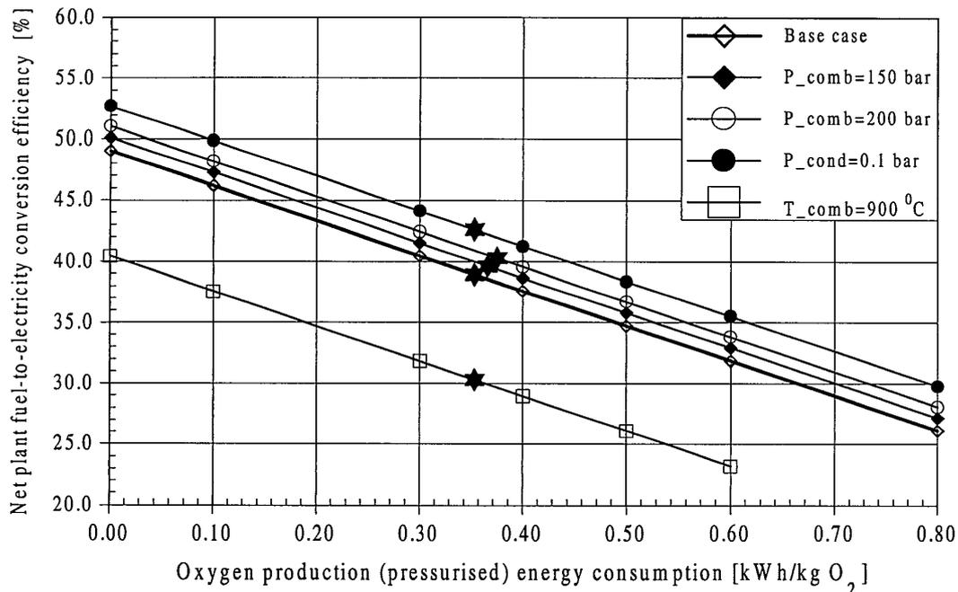
*Figure 2* Fuel-to-electricity conversion efficiency. The stars indicate the calculated points in the present study.
