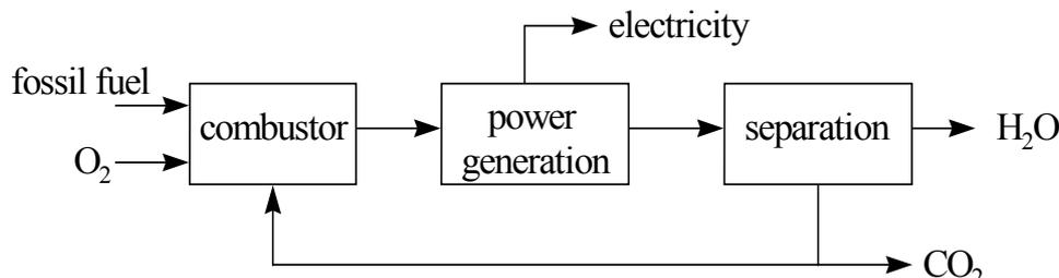
The gas leaving the combustor is typically >85%CO<sub>2</sub> by volume and the balance is steam (apart from excess oxygen and any impurities introduced by the fossil fuel). Oxygen is normally assumed to be obtained by cryogenic air separation (ASU)<sup>2</sup> but there are other options such as pressure swing absorption (PSA).
