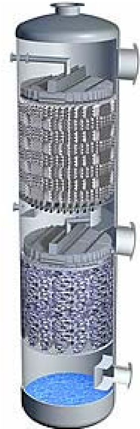
Packed column, example (distillation)
