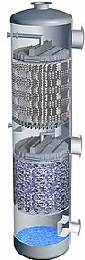
Packed column, example (distillation)
