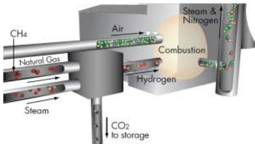
Figure 1 Before burning - Pre-combustion capture
