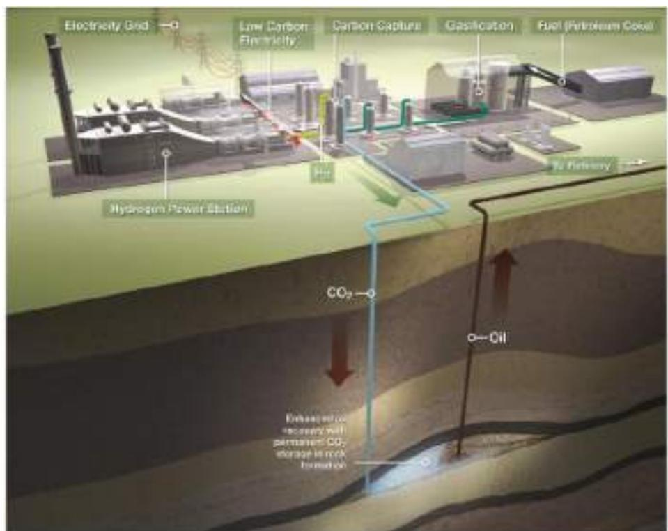
Figure 9 Illustration of a planned power plant in California with CCS. Illustration courtesy of BP and Edison Mission Group)
