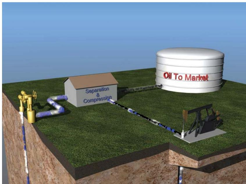
Water (blue) and CO<sub>2</sub> (white) are compressed and injected into oil reservoirs for enhanced oil recovery. Roughly 30% of the CO<sub>2</sub> returns to the surface with the oil (black), where it is separated and recycled.
