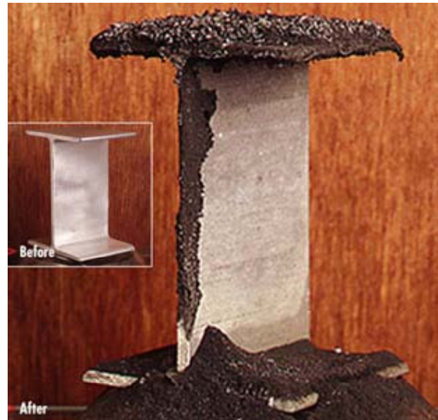
Figure 1: A small amount of mercury attacking an aluminium beam in less than an hour [courtesy of Popular Science website].
