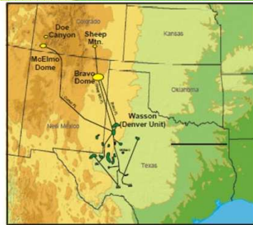
CO 2 flooding in the Permian Basin demonstrating CO 2 sources (yellow), flooded oil fields (green) and associated transmission lines.
