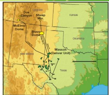
CO<sub>2</sub> flooding in the Permian Basin demonstrating CO<sub>2</sub> sources (yellow), flooded oil fields (green) and associated transmission lines.
