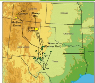
CO 2 flooding in the Permian Basin demonstrating CO 2 sources (yellow), flooded oil fields (green) and associated transmission lines.
