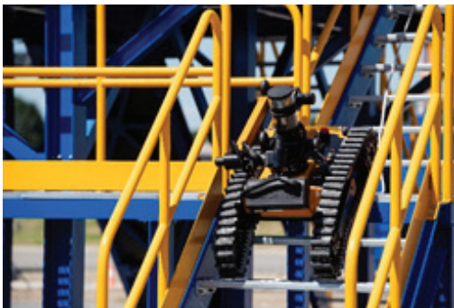
Inspection robot in stairs
