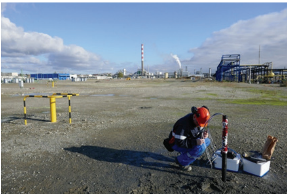
Velocity measurement of groundwater flow at ADYCHATS with innovative velocity probes
