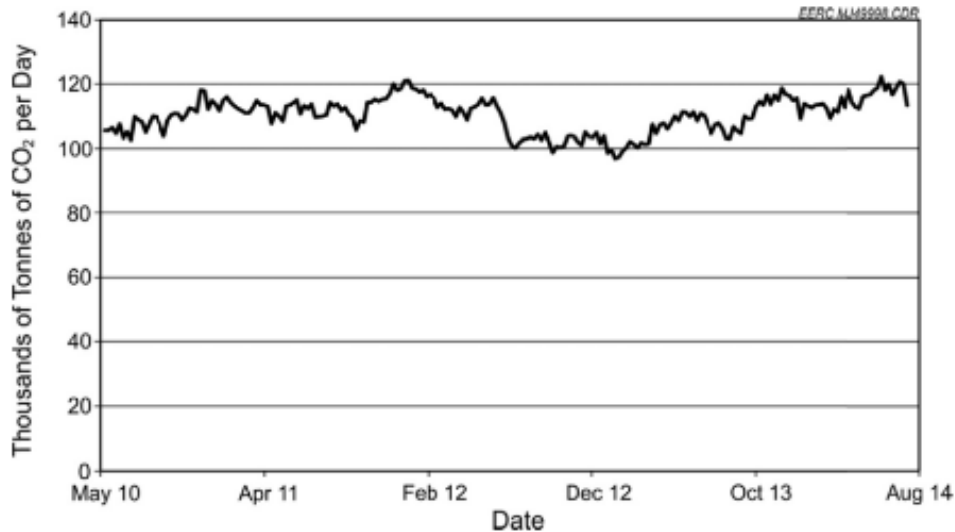
Figure 3. Variability in weekly CO 2 emissions from the production of ethanol fuel in the United States in 2014 22 .
